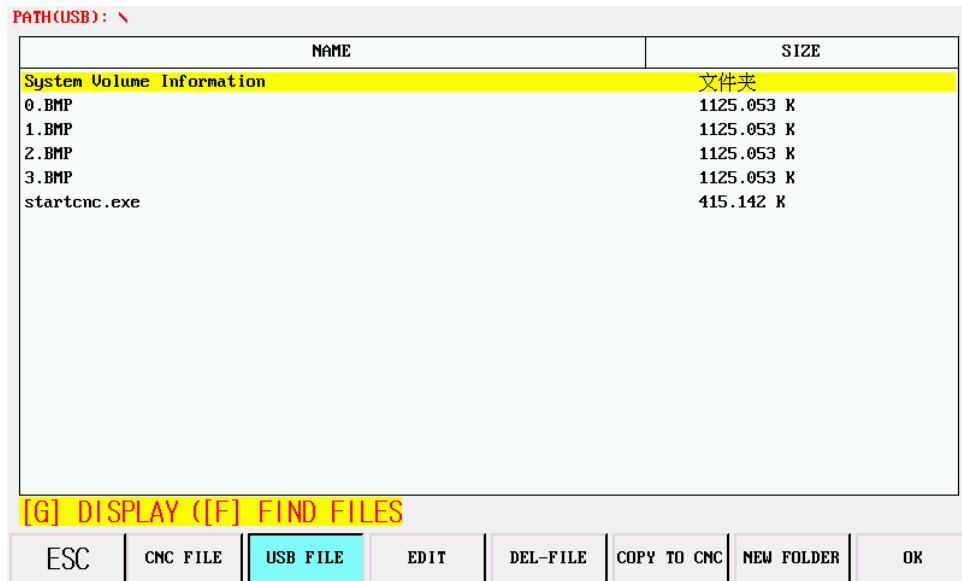
Under the file management interface, press 【 F2】 into the Usb file interface, in the interface, 【 F5】 Automatically from the "copy to usb flash drive" into "copy to the native". In the choice to the corresponding cutting code file, press 【 F5】 the system will automatically save the file to the file.
