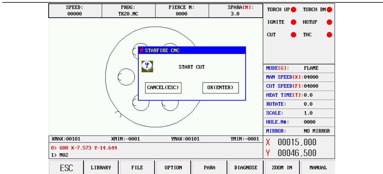
At this point, press the Start automatic processing, press Exit the processing, Back to the main interface
