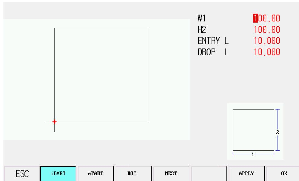
Press the direction key **【↑】**【↓】**【←】**【→】**** Move highlighting the cursor, modify graphics parameters, Press **[F1] - [F4]** Choose graphically, Rotation discharge. Press **[F6]** Submit the modified parameters, Press **[F7]** Confirm the cutting current graphics, Confirmed the system automatically returns to the switch on the main interface, and displays the graphics editor.****
