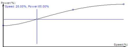
As shown below, if the laser power is 500W, after setting the cutting speed to be 100mm/s, peak current to be 90% and cutting power to be 80%, when the actual cutting speed drops down to 40mm/s, namely the red marker point, the power of laser is as follows:
