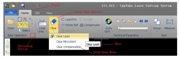
The whole toolbar is divided into four "pages", which can be selected by the four menus "Start", "Drawing", "Numerical control" and "View". When selecting text and other special objects, the pages related to the selected contents will appear. Furthermore, the page "Being Processed" will appear
