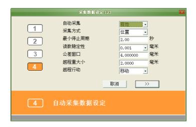
Wherein, please set and record the minimum value of the stop cycle, which will be used when setting parameters in CypCut. After completion, the laser interferometer begin to collect data.
