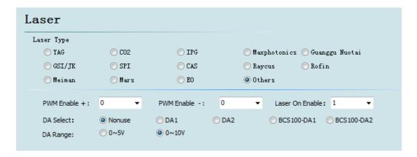
**Laser On Enable:** Correspond to the shutter button on software, this signal can open shutter of the laser.
