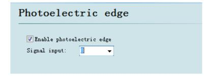
This function applies Omron E3Z-L61-type diffuse optical switch. The effective detection range of the optical switch is 90 ~ 120mm. Automatic seeking edge can be achieved by optical edge seeking, whose speed and precision is higher than capacitance edge seeking. After click this function and configure the input port of corresponding optical switch, you can use optical edge seeking in CypCut software.
