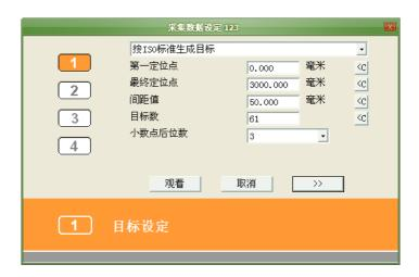
The first anchor point is always 0, and final positioning point is the stroke range. The interval value is the preceding measurement interval.
