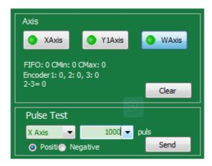
3. If the pulse feedback transmitted forward is negative, enter "the platform configuration tool - Machine page" to reverse the encoder corresponding to the number of axis. (Note: Have to set synchronously the encoder feedback of the second shaft and the third shaft in case of double-drive machine).
