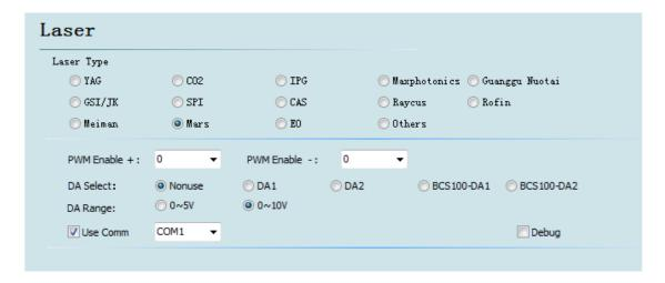
Except remote control, the configuration of Mars, Raycus and SPI fiber laser is the same as IPG fiber laser, and supports serial port communication.
